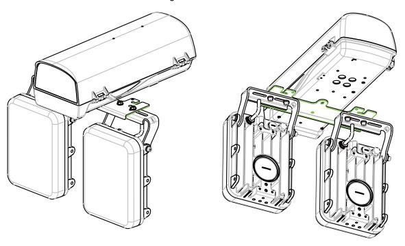
4. Adjust the illuminators' tilt angles if necessary.
