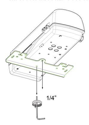
3. Secure two illuminators to the mounting bracket.
