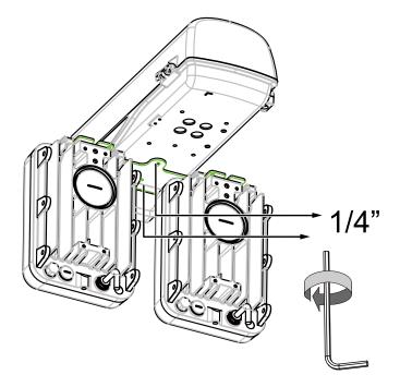
3. Use the different holes indicated below for installing 2 illuminators.
