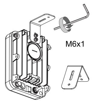
2. Secure the illuminator to the bottom of enclosure.
