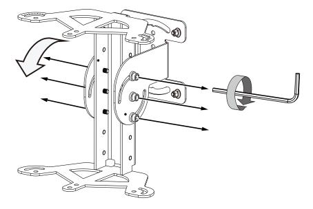
3. Secure the illuminators to the brackets using 4 included hex socket screws. If preferred, you can turn the illuminators to be facing outwards to avoid over-lapping the IR light coverage areas.
