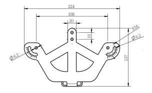
1. Install the base plate directly to a wall, to a pole-mount, or to a corner-mount bracket. Refer to the Installation Guide that came with the mounting brackets for more information.
