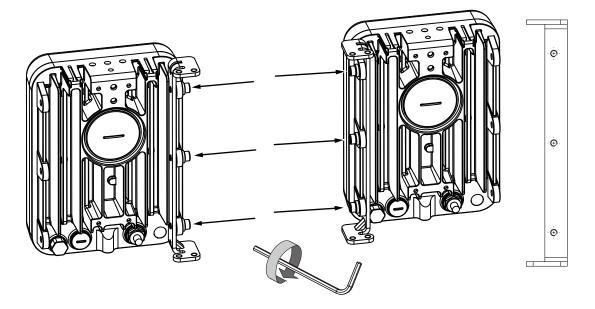
3. Secure two illuminators to the sides of B05 mounting bracket, each using 4 M6 socket screws.
