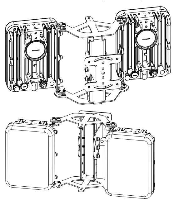
4. Install another illuminator to the center. Adjust the pan and tilt angles if preferred.
