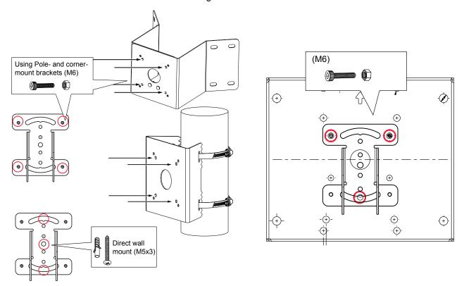
2. Secure the retention bracket to the base plate using 6 M6 socket screws. You can tilt its angle while doing it.
